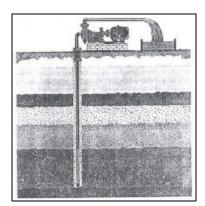
It consists of a bore hole built into ground with the purpose of tapping ground water from porous zones. In sedimentary formations
